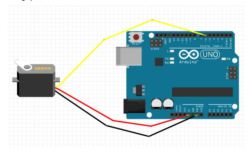
A servo wiring diagram
