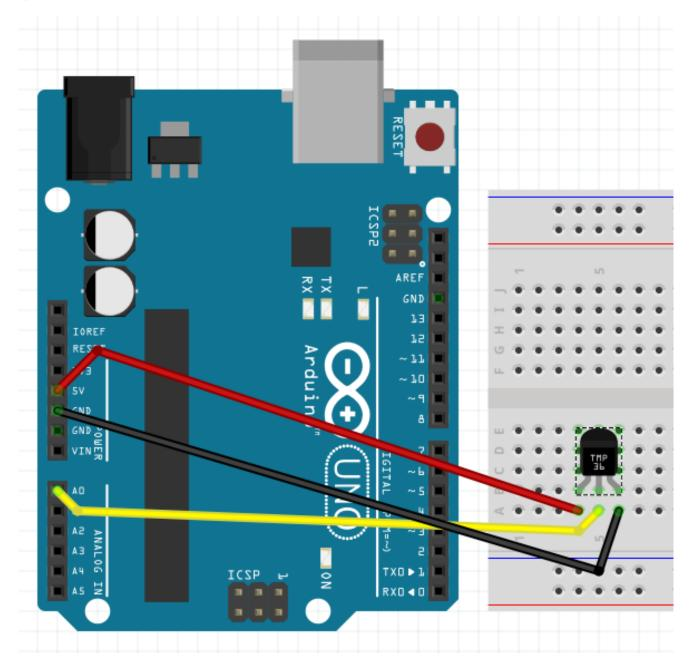
Wiring up the temperature sensor
