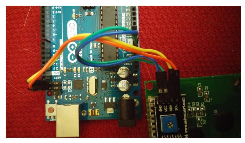
Photo of i2c backpack wiring. Wiring up regular LCDs
