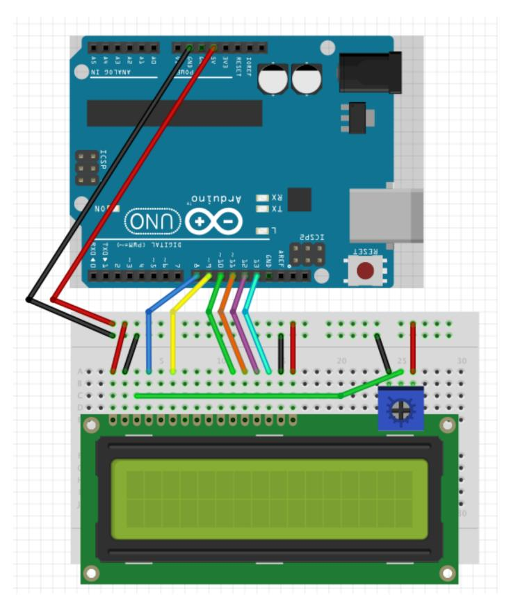
Wiring diagram—regular LCD
