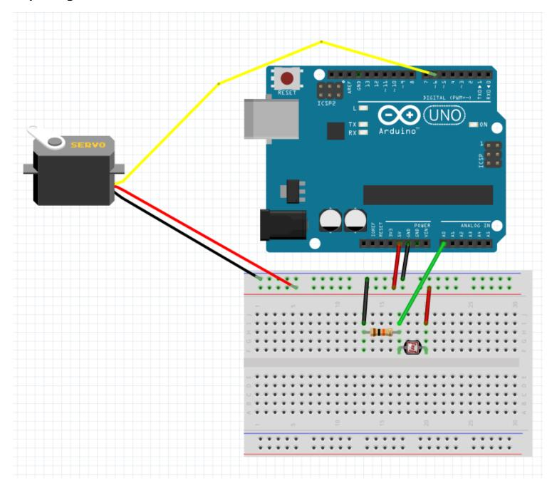
A servo and photoresistor wiring diagram
