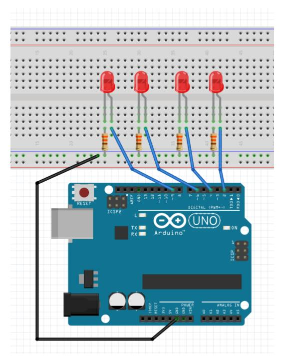
Wiring for our multiple LEDs project
