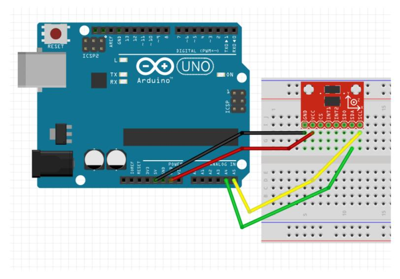
Accelerometer wiring for NON-R3 Arduino Uno
