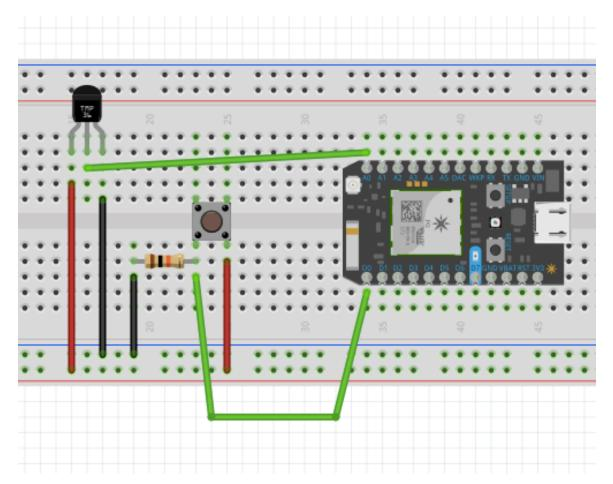
A WeatherBot Photon Schematic
