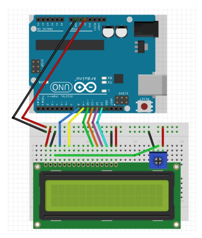
Wiring up a non-i2c LCD
