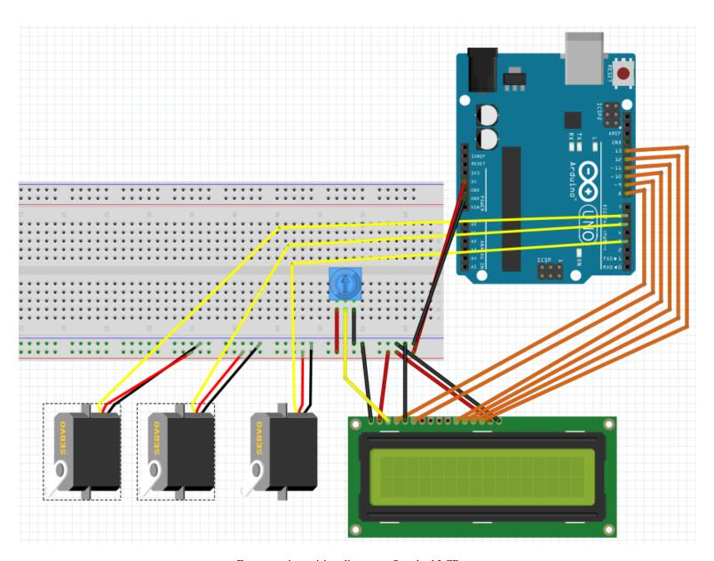
Events project wiring diagram—Standard LCD
