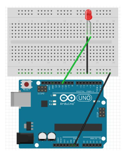
Wiring an LED with a breadboard
