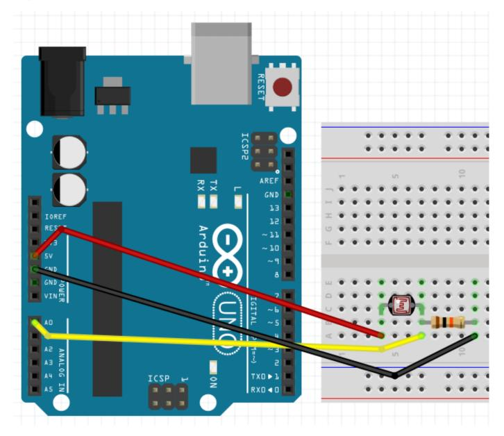
The wiring diagram for the photocell
