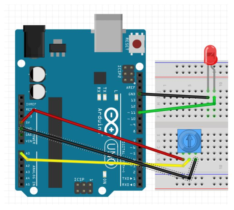
Wiring diagram for a dimmer switchCoding our dimmer switch
