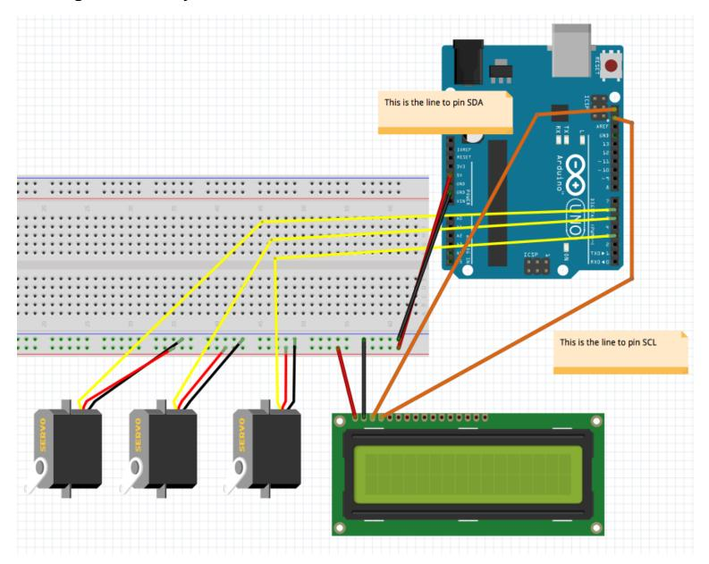
Events project wiring diagram—i2c LCD
