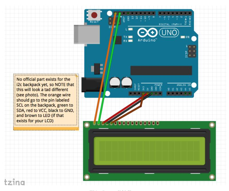
Wiring diagram—I2C LCD
