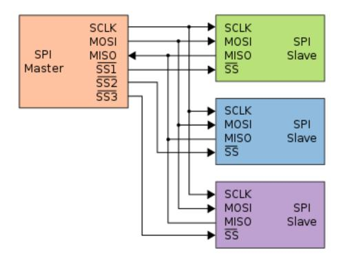
The SPI explained—Image credit https://en.wikipedia.org/wiki/Serial\_Peripheral\_Interface\_Bus
