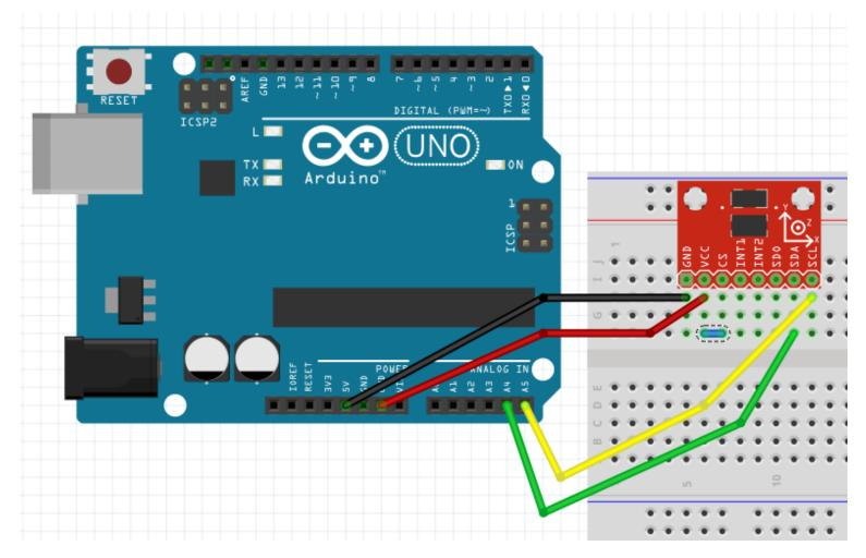
Wiring for the SparkFun breakout board
